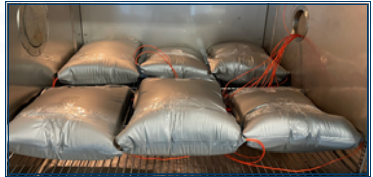
TempAid CRT Mailers are qualified in our ISTA Certified Laboratory for temperature stability, comparative R value testing, and thermal modeling
